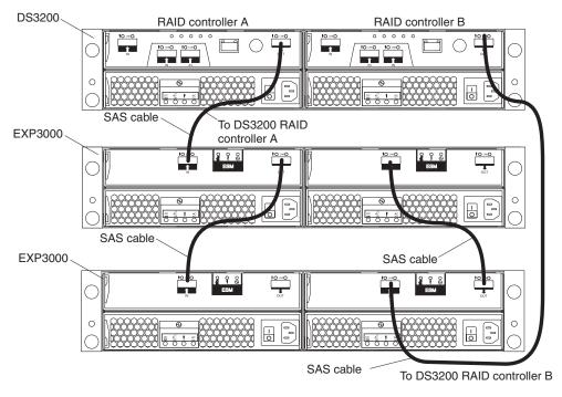
Figure 21. One dual-controller DS3200 and two storage expansion enclosures
